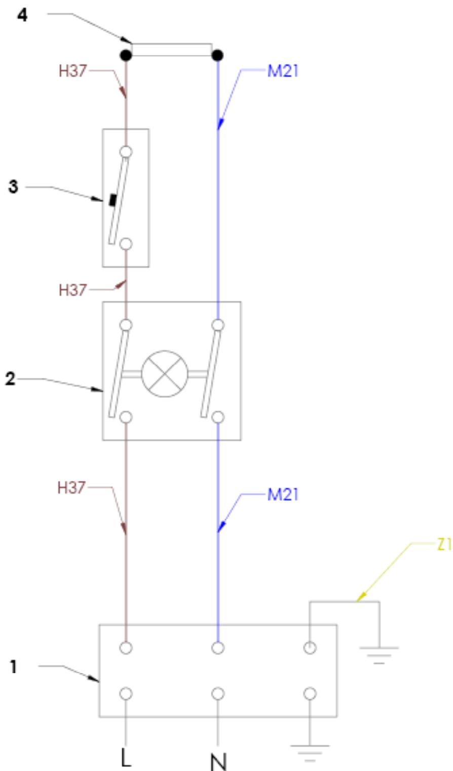
**EL. CONNECTION DIAGRAM / SCHALTPLAN / SCHÉMA DU ELECTRIQUE**
